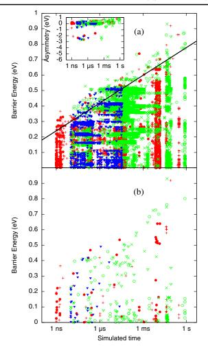
FIG. 3 (color online). (a) Energy barrier of all executed k-ART events. Points above the solid black line correspond to the 10% highest energy barriers in each time frame. Inset: Potential energy asymmetry (final energy minus initial energy) of the executed events with an energy barrier lying in the top 10% of the barriers plotted in (a) for each time frame. (b) Energy barrier of the k-ART events that release at least 0.5 eV of heat.
