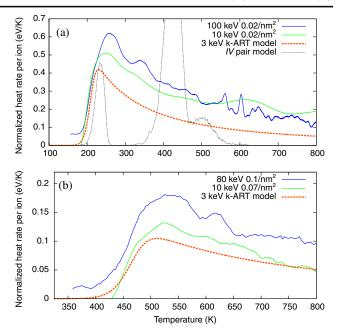
FIG. 1 (color online). Heat release as a function of temperature starting from (a) liquid nitrogen (LN) and (b) at room temperature. Solid lines: Experimental results; the NC signals are divided by the number of implanted ions and scaled to 3 keV (see text). Dashed red lines: Model derived from k-ART after 3 keV Si ion implantations. Dotted black curve: Simulation based on the *IV*-pair model at LN temperature.
