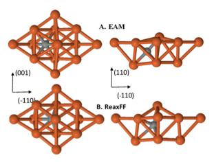
**Figure 4** Most stable structure for a carbon atom in the Fe(110) subsurface calculated using the EAM (A) and using the the ReaxFF (B). Brown: Fe atoms, grey: carbon atom. Fe–Fe (brown) and Fe–C (brown–grey) bonds are also shown.
