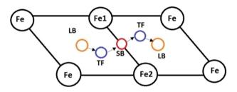
**Figure 9** Migration path of carbon on the Fe(110) surface predicted by the NEB method using the EAM and DFT. The C atom migrates between LB sites (yellow circle) by crossing a barrier at the SB site (red circle) and local minima at the TF sites (blue circle) on the way.
