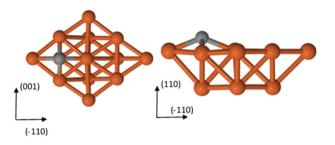
**Figure 3** Most stable structure (LB) of carbon on a Fe(110) surface calculated using the EAM and the ReaxFF, where the EAM puts the carbon at a slightly higher position than the ReaxFF or DFT. Brown: Fe atoms, grey: carbon atom. Only surface with  $(4 \times 4)$  cells are shown.
