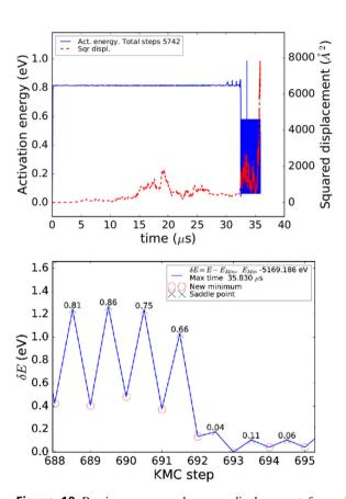
**Figure 10** Barrier energy and square displacement for carbon diffusion from bulk to surface predicted by k-ART at 600 K, as a function of time (top). A close-up view of the energy profile is shown with respect to the KMC steps as the carbon atom emerges from the bulk onto the surface (bottom).
