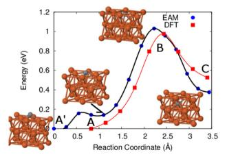
**Figure 6** Minimum energy path of carbon diffusion through Fe(110) surface into subsurface calculated by using the NEB method with the EAM potential and the DFT. The reaction coordinate of the DFT is shifted so that its initial image is located at the same coordinate as image A of the EAM.
