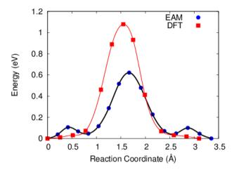
**Figure 8** Minimum energy path of carbon diffusion over the Fe(110) surface calculated using the NEB method with the EAM potential and DFT.
