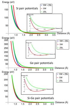
Fig. 2. SW pair potential, ZBL and the combination of the two potentials (SW + ZBL) as described above for Si-Si interaction, Ge-Ge and Si-Ge. Zooms on the plots between 1.5 Å and 3.0 Å are inserted. On the zooms, SW and SW+ZBL curves are completely equal.
