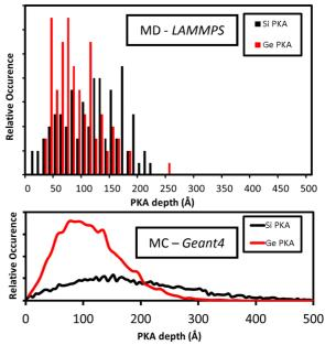
Fig. 13. PKA penetration depth distribution in Si<sub>0.8</sub>Ge<sub>0.2</sub> starting from 10 keV Si and Ge PKA obtained with *LAMMPS* and *Geant4*.
