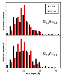
Fig. 12. Penetration depth of Si and Ge 1 keV PKA in  $Si_{0.8}Ge_{0.2}$  and  $Si_{0.7}Ge_{0.3}$ . 300 simulations per PKA types were performed.
