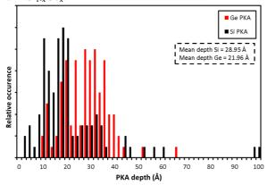
Fig. 9. Penetration depth of 1 keV Si and Ge PKA in Si<sub>0.8</sub>Ge<sub>0.2</sub>. Simulations were performed with SW potential only.
