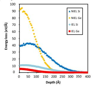
Fig. 8. Non Ionizing Energy Loss (NIEL) and Ionizing Energy Loss (IEL) of  $10~\rm keV$  Si and Ge PKAs in  $\rm Si_{0.8}Ge_{0.2}$  versus depth. The calculations have been performed on  $10000~\rm cascades$  for each PKA type with SRIM.
