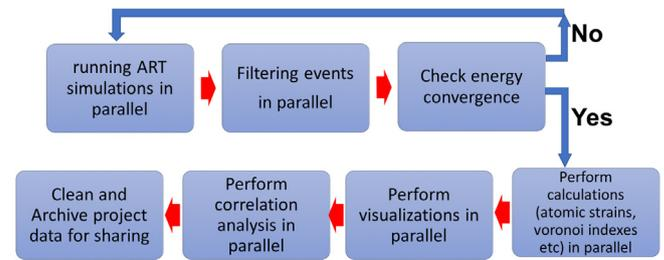
**Fig. 1.** The pipeline software architecture of this ART\_data\_analyzer package allows user customization in running various module tasks in a standard workflow.
